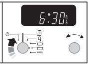
Set the oven(s) to the cooking temperature you need (don't forget to set a function if using the Multi-function oven).
